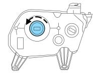
**WARNING:** Handle a halogen headlamp bulb carefully and keep out of children's reach. Grasp the bulb only by its plastic base and do not touch the glass. The oil from your hand could cause the bulb to break the next time the headlamps are operated.
